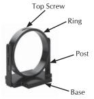
3. If the ScreenStar lens is not directly in the center of the prime lens, you will need to adjust the height and tilt. Loosen the two (2) Allen screws on each side of the posts in order to slide the ScreenStar lens up/down. Tilt the ring to angle the lens. Tighten the Allen screws to secure the lens into place.
