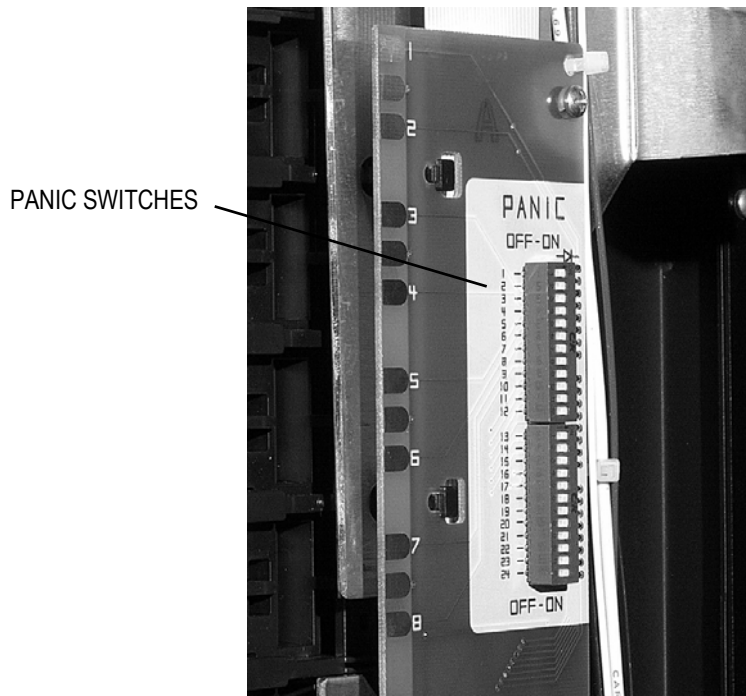
Figure 9 - Panic Switch Location (typical)
