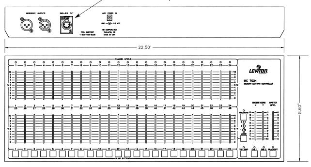
The MC 7000 Series lighting consoles are simple and flexible with three operating modes. These consoles provide standard 2-scene preset operation, single scene wide mode for double channel capacity and memory scene operation mode.
