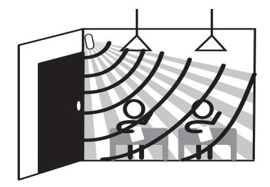
The versatile OSW12-M Occupancy Sensor can be mounted on the wall to provide full room coverage when low-hanging lights or other obstacles are present. Infrared and ultrasonic signals are used for maximum reliability.
