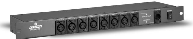
The DMXSM-H18 splits a single DMX 512 channel DMX input into (8) completely isolated 512 channel DMX outputs. Perfect for segregating automated devices from conventional lighting or when an alternative to the traditional daisy-chained signal routing is desired.
