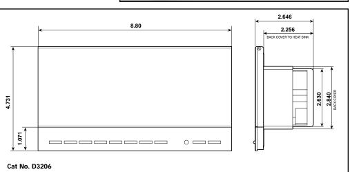
LCD displays the exact zone light level so that repeatable settings can be achieved. The D3206 provides eight different scene buttons; the active scene button will remain lit. Once scenes are programmed, any zone may be individually dimmed or brightened without affecting the rest of the scene. A number of other helpful pushbuttons round out the functionality: group dim, group brighten, maximum brightness, and off.
