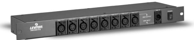
The DMXSM-H18 splits a single DMX 512 channel DMX input into (8) completely isolated 512 channel DMX outputs. Perfect for segregating automated devices from conventional lighting or when an alternative to the traditional daisy-chained signal routing is desired.
