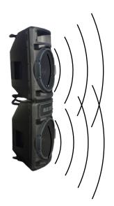
In a setup were the sub is on the floor and a M•Flex 15 is placed on top of it, you can choose to have the High pass selector off. Then both the Sub and the M•Flex 15 receive the same frequency and support each other.
