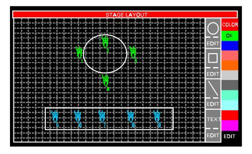
All the fixtures, lines and texts placed on this screen, will appear also in the stage layout of the main program. There are 2 stage layouts (page 1 of fixtures 1-70 and page 2 of fixtures 71-140). Note : In previous software versions only 20 different types of fixtures could be selected. From version 6.2 it is increased to 40.
