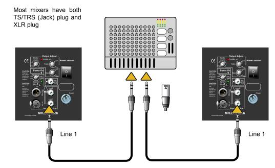
Stereo setup with either four M•Flex 12 or four M•Flex 15 and a mixer
