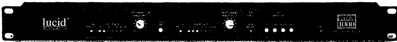
Lucid Technology's ADA1000 provides two independent input channels that can be linked for stereo operation.
