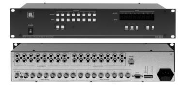
The **vs-626**, **vs-824**, and **vs-828** are high performance matrix switchers for composite video and unbalanced stereo audio signals. Switching during the vertical interval ensures glitch-free switching with genlocked sources.
