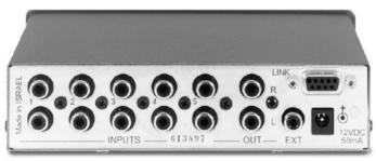
The VS-55A is high performance switcher for unbalanced stereo audio signals. It switches any one of five signals to a single output.
