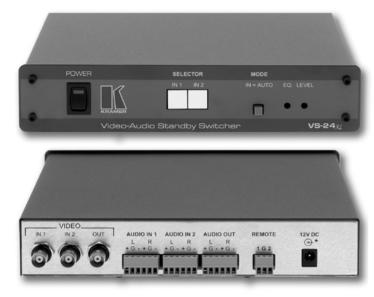
The VS-24×I is a high performance switcher for composite and balanced stereo audio signals. When configured as a stand-by switcher, it will switch to input 2 when the input 1 signal is interrupted.
