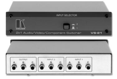
The VS-21 switches three identical channels simultaneously. It can serve as a high performance switcher for component video (YUV or RGB) signals. It switches any one of two component signals to a single component output. The VS-21 can also switch composite video with two audio channels, three independent composite video channels or any other combination.
