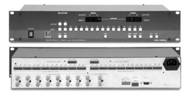
The VS-1002xI, VS-1202xI, and VS-1602xI are high performance matrix switchers for composite video and balanced stereo audio signals. Switching during the vertical interval ensures glitch-free switching with genlocked sources.
