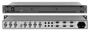
The VP-72 is a seven input multi-format distribution amplifier for composite, s-Video, component (HDTV), and computer graphics video signals with resolutions ranging from VGA through UXGA and higher. It was designed from user feedback to complement Kramer's  $ProScale^{TM}$ digital scaler/switcher line and includes seven 1:2 distribution amplifiers in one package: two composite, two s-Video (Y/C), one component, and two computer graphics video.
