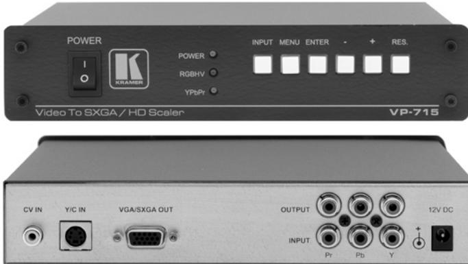
The **VP-715** is a digital scaler for composite video, s-Video (Y/C), and component video (YUV) signals. It will scale a video signal to a selectable computer graphics video or HDTV output.
