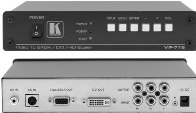
The **VP-716** is a digital scaler for composite video, s-Video (Y/C), and component video (YUV) signals. It will scale a video signal to a selectable computer graphics video or HDTV output.
