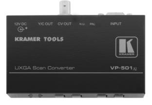
The **VP-501**×I is a scan converter for computer graphics video signals. It converts computer graphics video signals up to UXGA (1600 x 1200) to composite and s-Video (Y/C) signals simultaneously in either PAL or NTSC formats.
