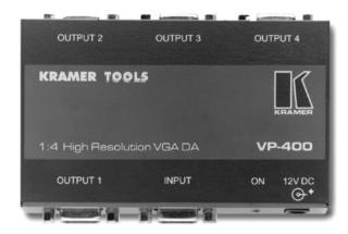
The VP-400 is a high performance distribution amplifier for computer graphics video signals with resolutions ranging from VGA through UXGA and higher. It takes one input, provides correct buffering and isolation, and distributes the signal to four identical outputs.
