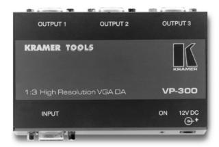
The VP-300 is a high performance distribution amplifier for computer graphics video signals with resolutions ranging from VGA through UXGA and higher. It takes one input, provides correct buffering and isolation, and distributes the signal to three identical outputs.
