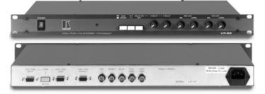
The **VP-22** is a high performance computer graphics video processor, line, and distribution amplifier for computer graphics video signals with resolutions ranging from VGA through UXGA and higher. It takes one input, provides correct buffering and isolation, and distributes the signal to one HD15 and one set of 5-BNC output.
