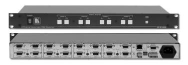
The VP-214DS is a machine with four computer graphics switchers in one box. When configured as a standby switcher, each 2x1 switcher will switch to the secondary input upon loss of the primary input.
