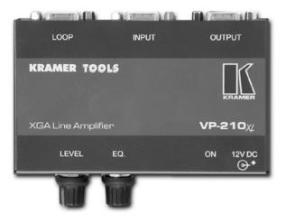
The VP-210xI is a high performance line amplifier for computer graphics video signals with resolutions ranging from VGA through UXGA and higher. It provides controls to compensate for signal losses inherent in long cable runs.
