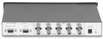
The VP-103 is a line amplifier and format converter for computer graphics video signals. It accepts a computer graphics video input on a 15-pin HD connector and converts it to two identical outputs of either RGBS, RGsB, or RGBHV.
