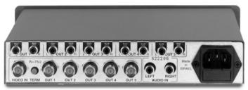
The Kramer VM-5S is a high performance distribution amplifier for composite or SDI video and unbalanced stereo audio signals. It will take one input, provide correct buffering and isolation and distribute the signal to 5 identical outputs.
