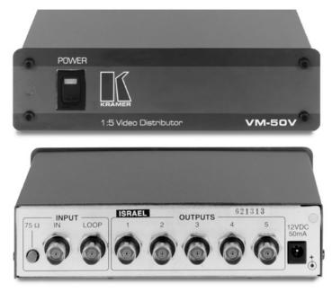
The Kramer VM-50V is a high performance distribution amplifier for composite or SDI signals. It takes one input, provides correct buffering and isolation, and distributes the signal to five identical outputs.
