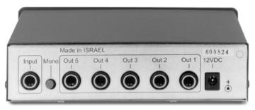
The Kramer VM-50H is a high performance distribution amplifier for Headphone signals. It takes one stereo headphone input and distributes the signal to five identical stereo headphone outputs.
