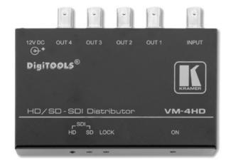
The **VM-4HD** is a high performance distribution amplifier for SDI (SMPTE 259M and SMPTE 344M) and HD-SDI (SMPTE 292M) signals. It takes one input, provides reclocking and equalization and distributes the signal to four identical outputs.
