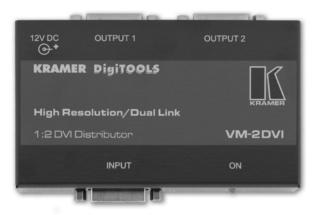
The VM-2DVI is a distribution amplifier for DVI-D video signals. It takes one input and distributes the signal to two identical outputs. Use Kramer \dual Link DVI cables for best
