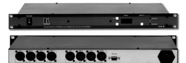
The VA-4 is a volume controller for two channels of balanced stereo audio signals on XLR connectors. The volume of each stereo channel can be adjusted independently of the other stereo channel.
