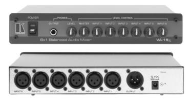
The VA-15xI is a 6 channel mixer for mono balanced audio signals on XLR connectors. It inputs 6 channels of any combination of line or microphone level audio signals to a balanced mixed audio and a headphone signal output.
