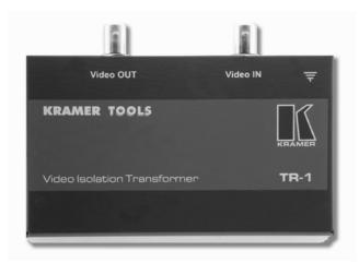
The TR-1 is a high resolution video isolation transformer for composite video signals. It provides complete isolation between devices thus eliminating video hum, ground loops, and DC offsets which can degrade picture quality.
