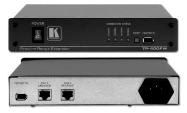
The **TP-400FW** is a twisted pair transmitter or receiver for FireWire (IEEE 1394) signals. When used in pairs, one will convert a FireWire signal into a twisted pair signal and the other will convert the twisted pair back to a FireWire signal and simultaneously output the twisted pair signal to another **TP-400FW**.
