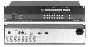
The **SD-7388** is a high performance matrix switcher for SDI (SMPTE 259M) video signals. Switching during the vertical interval ensures glitch-free switching with genlocked sources.
