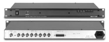
The SD-7108 is a high performance distribution amplifier for multistandard SDI (SMPTE 259M) video signals. It takes one input, provides reclocking and equalization and distributes the signal to eight identical outputs and one parallel ECL output.
