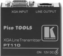
The **PT110** is a twisted pair transmitter for computer graphics video signals. It converts a computer graphics signal into a twisted pair signal which will be converted back to a computer graphics video signal when used in conjunction with the Kramer TP-120 twisted pair receiver (or other compatible Kramer receiver).
