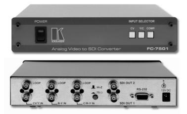
The **FC-7501** is a format converter for composite video, s-Video or component video (YUV) signals. It converts either PAL, SECAM, and NTSC composite video, s-Video, or component (YUV) signals into 2 SDI (SMPTE 259) signals simultaneously.
