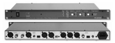
The FC-2000 MultiCoder is a broadcast quality universal transcoder for analog and digital audio signals. It simultaneously converts between any of the most popular digital and analog audio formats and sampling rates.
