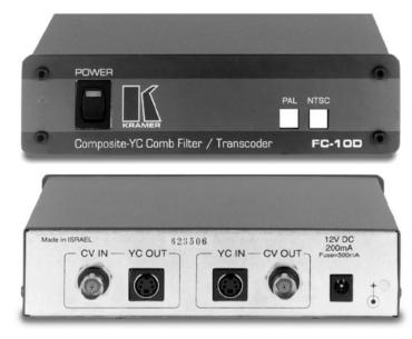
The FC-10D is a high performance bi-directional transcoder for composite and s-Video (Y/C) signals. It simultaneously converts a composite video input to an s-Video output through a digital comb filter, and an s-Video (Y/C) input to a composite video output.
