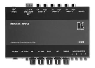
The 903 is a high performance integrated personal stereo amplifier for unbalanced stereo signals. It allows selection between four inputs and delivers a speaker output of 10 watts RMS power per channel into a 4 ohm load.
