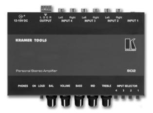
The 902 is a high performance integrated personal stereo amplifier for unbalanced stereo signals. It allows selection between four inputs and delivers a speaker output of 4.5 watts RMS power per channel into a 4 ohm load.
