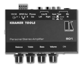
The **901** is a high performance integrated personal stereo amplifier for unbalanced stereo signals. It accepts a stereo audio signal and delivers a speaker output of 2 watts RMS power per channel into a 4 ohm load.
