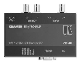
The **7508** is a multi-format converter for composite video or s-Video (Y/C) signals. It converts either PAL, SECAM, and NTSC composite or s-Video (Y/C) signals into 2 SDI video (SMPTE 259M) outputs simultaneously.
