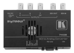
The 7408 is a format converter for SDI (SMPTE 259M) signals. It converts an SDI video signal to composite video, s-Video (Y/C), or component (YUV) video.
