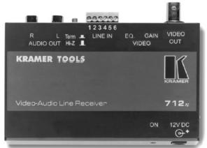
The 711xI and 712xI are a twisted pair transmitter and receiver for composite video and unbalanced stereo audio signals. The 711xI transmitter converts composite video and stereo audio to a twisted pair signal and the 712xI receiver converts the twisted pair signal back into composite video and stereo audio signals.
