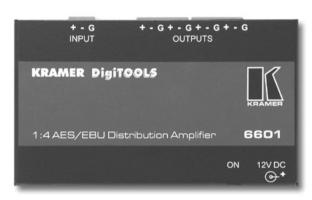
The **GGO1** is a high performance distribution amplifier for digital audio signals. It takes one input, provides reclocking and equalization and distributes the signal to four identical outputs.
