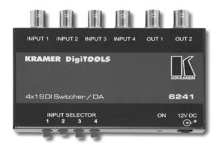
The **6241** is a high performance switcher for serial digital (SMPTE 259M) video signals. It takes any one input, provides reclocking and equalization and distributes the signal simultaneously to two identical outputs.
