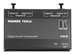
The 465 is a transcoder for AES/EBU and optical S/PDIF digital audio signals. It simultaneously converts AES/EBU to optical S/PDIF digital audio signals and optical S/PDIF to AES/EBU digital audio signals.
