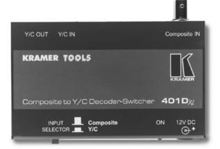
The 401DxI is a high performance format converter and switcher for composite video and s-Video signals. It switches one composite or one s-Video (Y/C) input to a single s-Video (Y/C) output.
